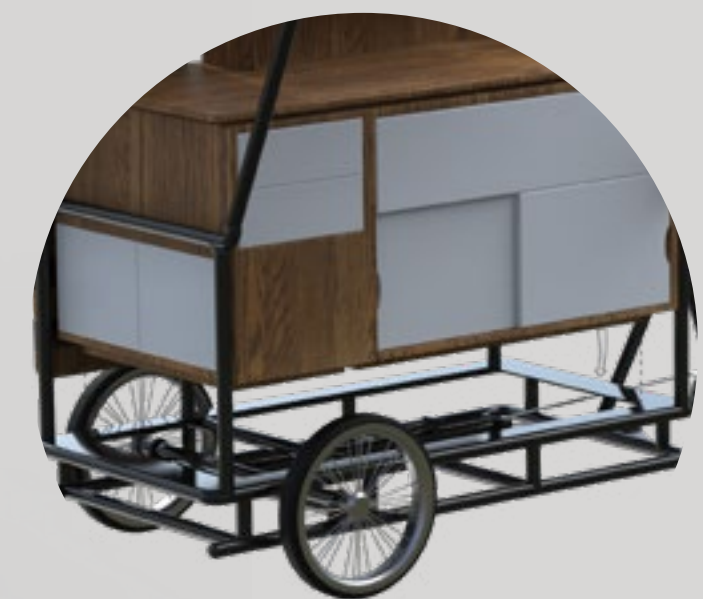
Cabinets are screwed to the frame from the bottom through the welded screw plates
