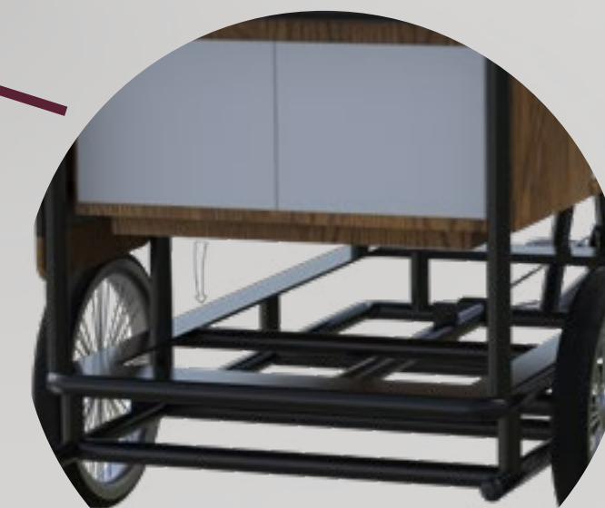
Cabinets are screwed to the frame from the bottom through the welded screw plates
